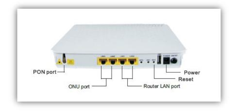
ONU-8081 (2GE+2FE) is an EPON user terminal, which meets the SOHO broadband access, FTTH broadband speed ,FFTH/FTTD of cable-television operator. The equipment based on mature, stable, cost-effective Gigabit EPON technology combines Gigabit Ethernet switching technology, WIFI. It has high reliability, ease of administration and good QOS. The technology performance meets the IEEE802.3ah, China Telecom EPON equipment technical requirements (V2.1) specification requirements.
